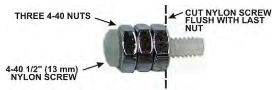
Figure 13. Cutting 1/2" (13mm) Nylon Screws.
