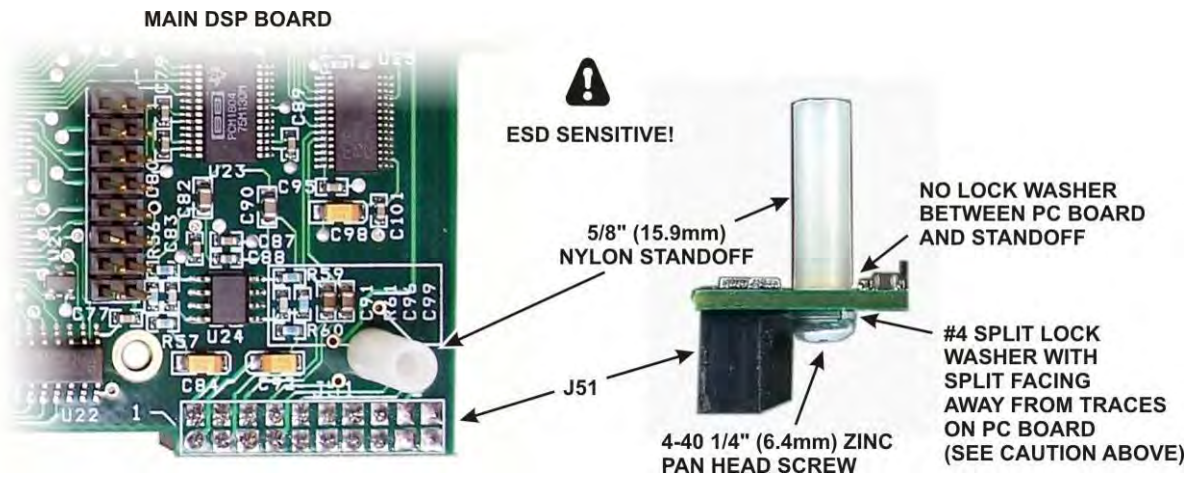
Figure 15. Installing Nylon Standoff on Main DSP Board.
