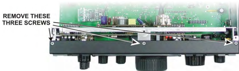
Figure 7. Removing Front Panel Mounting Screws.
