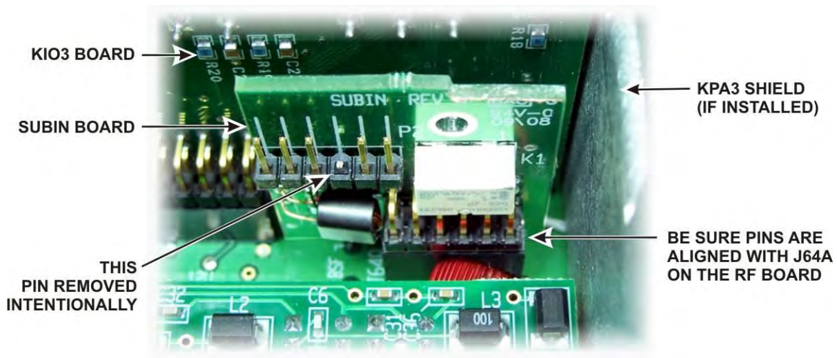
Figure 45. Mounting the SUBIN Interface Board.
