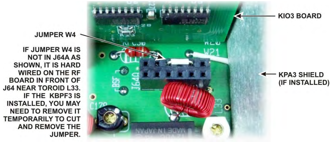
Figure 44. Jumper W4 on the K3 RF Board.
